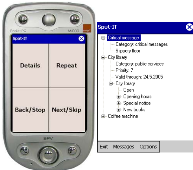
Figure 5. SPOT-IT user interface for the blind (left) and for the sighted (right).
